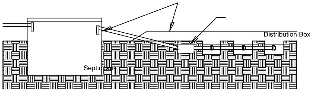
Note: Capping material must extend 10 ft. from trenches
